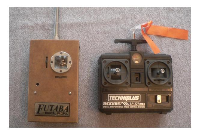
The transmitter on the left is a Futaba single stick 2 channel set. It could be used on rudder elevator or by fitting a ratchet rudder and motor. This was a very common way to fly in the 70s as radios were very expensive so 2 channel sets were very common.
